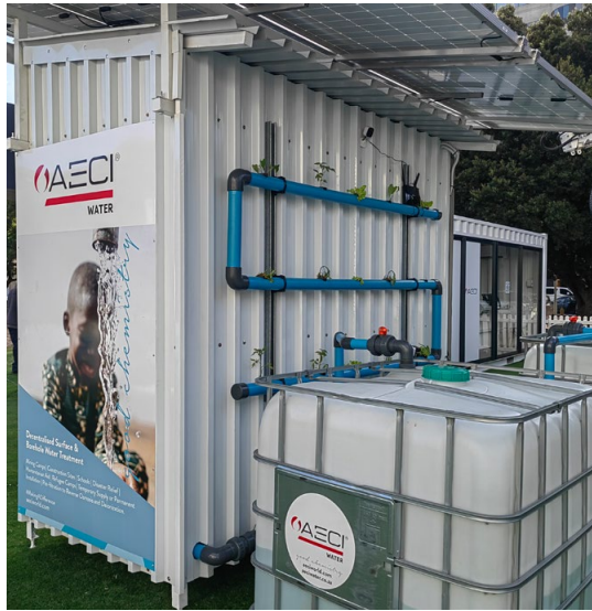
Decentralised Surface & Borehole Water Treatment Skid
